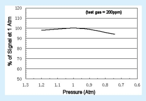
The Figure below represents the effect of altitude on the sensitivity of the NAP-505:
