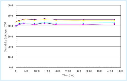
The sensors in this test were then stored in normal room condition to allow the electrolyte to re-establish a normal equilibrium. After a further 4 weeks in these conditions, the sensors were retested to confirm that the sensors had suffered no significant effect on their performance. The sensitivity signal of the sensors before and after the test is shown in the table below:
