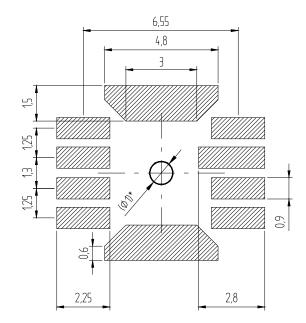
Recommended pad layout for soldering of the MS5201-XD on a printed circuit board
