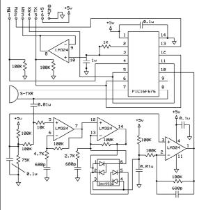
250mS after power-up, the LV-MaxSonar<sup>®</sup>-EZ2<sup>TM</sup> is ready to accept the RX command. If the RX pin is left open or held high, the sensor will first run a calibration cycle (49mS), and then it will take a range reading (49mS). After the power up delay, the first reading will take an additional ~100mS. Subsequent readings will take 49mS. The LV-MaxSonar<sup>®</sup>-EZ2<sup>TM</sup> checks the RX pin at the end of every cycle. Range data can be acquired once every 49mS.
