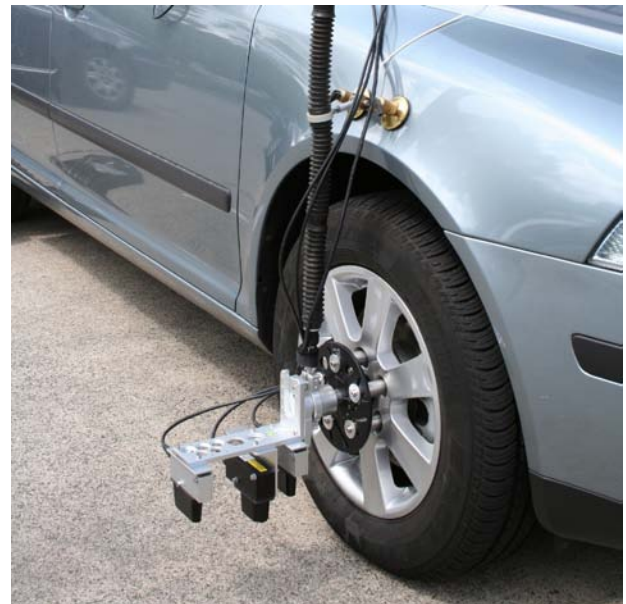
Fig. 2: A mounted DCA System (with optional SFII-P Sensor for measurement of tire slip angle)
