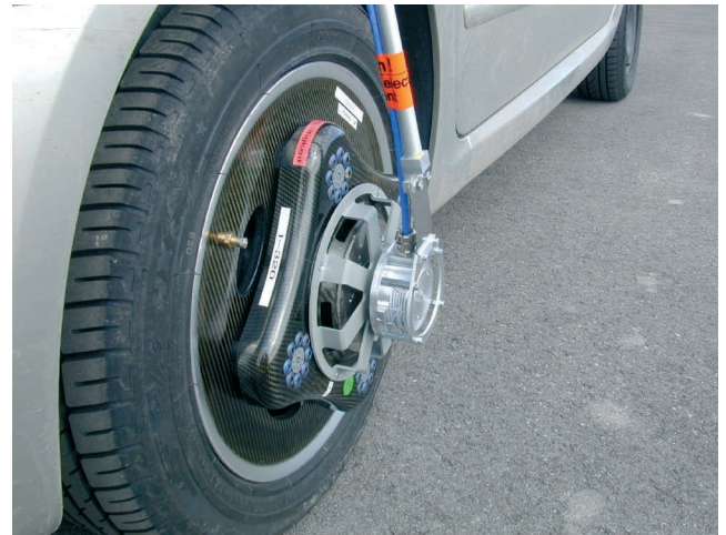
Fig. 1: Out-board transmission module on the RoaDyn® S625 System 2000 measuring wheel
