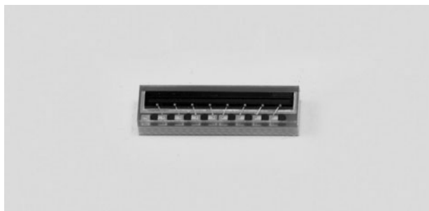
[Figure 2-2] COB example (S10226, unit: mm)
