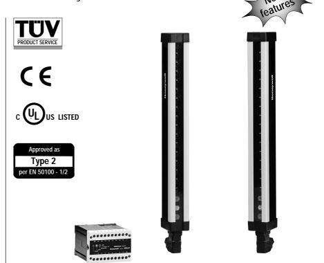
The FF-SLC curtain is an Electrosensitive Protective Equipement designed to protect operators of dangerous machinery. The safety light curtain detects any opaque object of a diameter greater than the resolution which interrupts the protected zone, the result being a stop signal sent to the machine. The FF-SLC series is an excellent alternative to traditional mechanical barriers, providing many benefits such as unobstructed working area, improved productivity, simple installation and maintenance.
