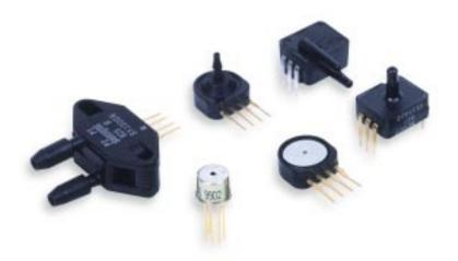
The SX Series of pressure sensors provide the lowest cost components for measuring pressures up to 150 psi. These sensors were specifically designed for use with non-corrosive, non-ionic media, such as air, dry gases, and the like. Convenient pressure ranges are available to measure differential, gauge, and absolute pressures from 0 to 1 psi (SX01) up to 0 to 150 psi (SX150).
