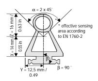
The low sensing surface at ends (70 mm) should not be used as detection surface. The highest actuating force applied on any point of the effective sensing surface should be less than 500 N.
