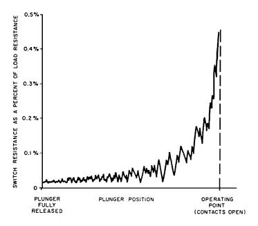
**Contact Resistance**: The resistance between a pair of closed contacts.
