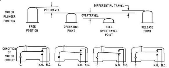
**Free Position:** Switch plunger is fully released and common contact is against normally closed contact.
