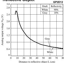
Fig.8 Analog Output Voltage vs.Detection Distance
