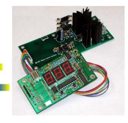
Designed for manufacturers of vehicular or other low voltage DC powered equipment, the Model 105 provides a cost-effective way to quickly and simply incorporate state of the art microprocessor based control capabilities into a wide variety of products. It precisely regulates electrically controlled thermal processes operating at temperatures between -9.9 and 99.9 degrees Celsius, typically maintaining temperature stability to well within  $\pm 0.1$  degrees of setpoint.
