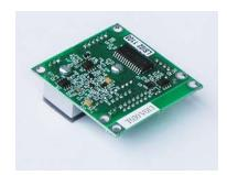
The *AirSense™* Model 305e's automated single gas verification makes field calibration a snap, and its superior design means significantly longer intervals between calibration. Technicians in the field can now easily calibrate the M305 simply by removing the port cap, plugging in the 2000 ppm cal gas (available from factory).
