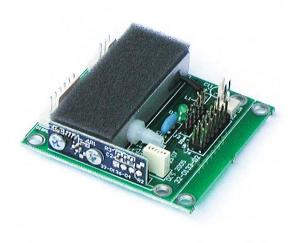
The AirSense™ Model 305e is a proven commercial non-dispersive infrared (NDIR) CO₂ concentration measurement subsystem designed for the OEM market: it provides equipment manufacturers the ability to integrate IR CO₂ sensing capability into a wide range of products. Specifically designed for embedded applications, the microprocessor-based Model 305 is the easiest and most cost-effective way to add CO₂ measurement to your product line.
