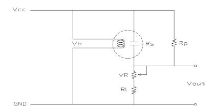
$\begin{array}{lll} Vcc : Circuit \ Voltage(5V) & Vh : Heater \ Voltage(5V) \\ R_L : Load \ Resistance & VR : Semi-Fixed \ Volume \\ \end{array}$
