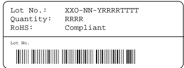
Figure 18: First label on reel: XX = Sensor Type (20 for SHT20), O = Output mode (D = Digital, P = PWM, S = SDM), NN = Chip Version, Y = last digit of year, RRRR = number of sensors on reel, TTTT = Traceability Code.
