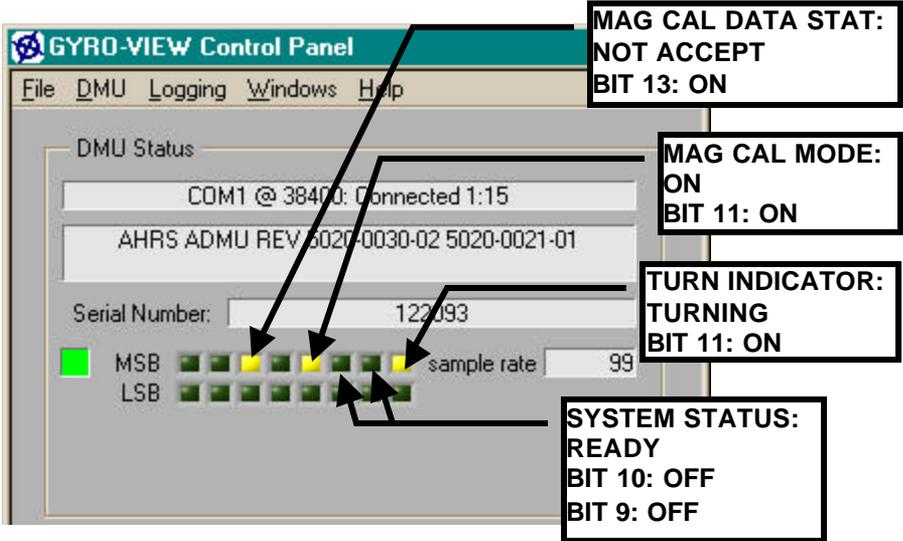
When the circle is completed, the following Gyro View BIT status should be displayed indicating the unit has made a full turn and is applying the estimated calibration. You should stop the rotation motion once the system status bits show the unit has reinitialized.
