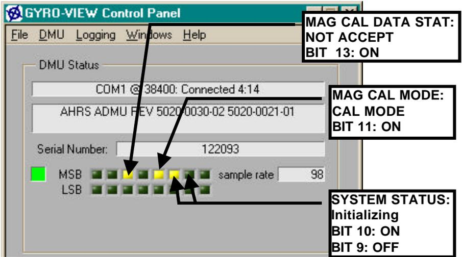
The Mag Cal Data Status Bit ON indicates that the compensation is not yet optimized and more calibration data needs to be collected. It won't usually signal a successful calibration after the first turn, unless the magnetic environment is extremely clean. Wait for the AHRS500GA to complete its initialization. At the end of the initialization, approximately 90 seconds, the following BIT status should be displayed:
