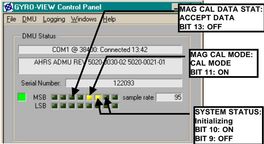
If the Mag Cal Data Status Bit is OFF as shown above, the data collected is adequate for the magnetometer calibration. No further aircraft motion is required. Proceed to the paragraph titled “ Completing the Calibration.”
