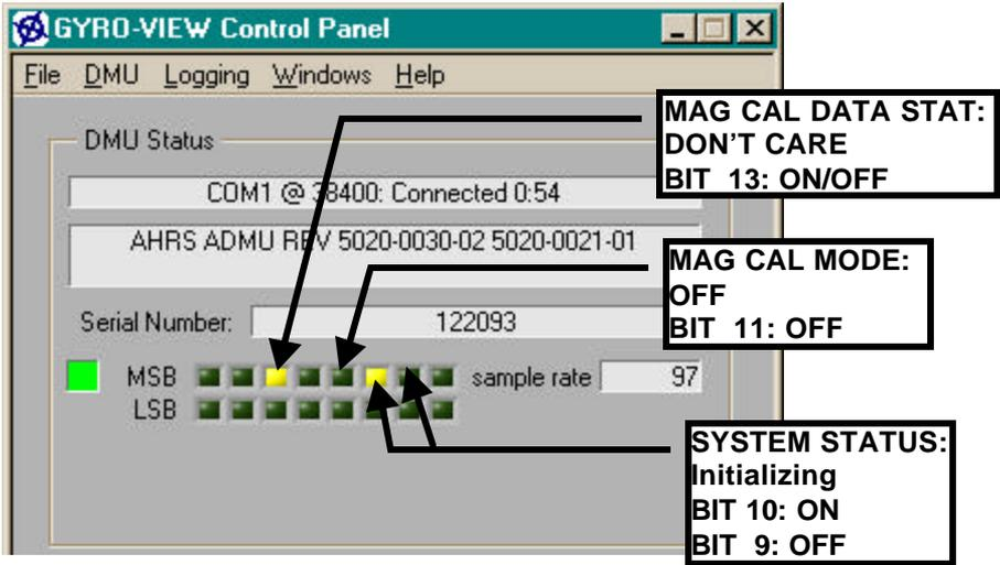
After approximately 90 seconds, the AHRS500GA will complete the initialization mode and change to the ready mode. At this time, the following BIT status should be displayed:
