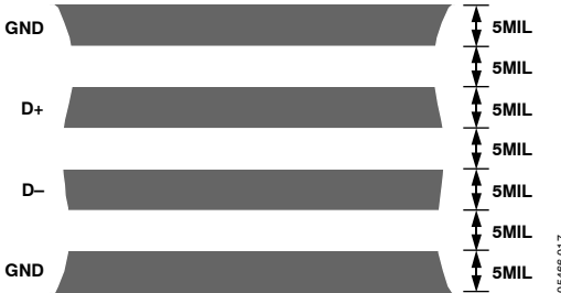
Figure 22. Typical Arrangement of Signal Tracks
