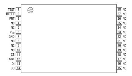
NC : No connection **28-Pin Plastic TSOP**
